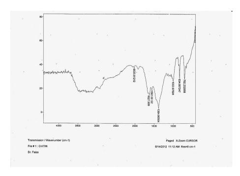
Fig 1: FTIR analysis of chitin purified from shrimp shells.
